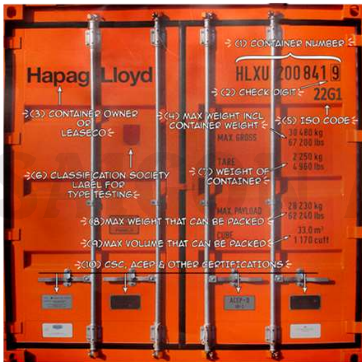
Markings on a Carrier Owned Container
